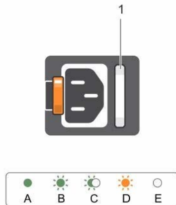
Figure 8. AC PSU status indicator
